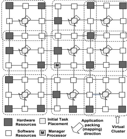
Fig. 3. Initial tasks placement for mapping applications
