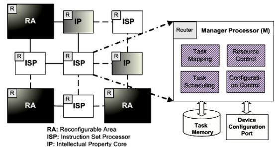
Fig. 1. Target MPSoC Architecture
